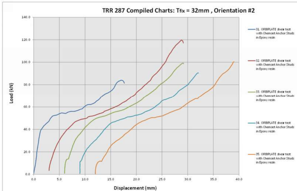
Shear Load vs Displacement Curve ORB2020PIAGH Rotational Horizontally aligned and bolt at extremity of slot 32mm plate thickness, M20 ChemSet Anchor Stud
