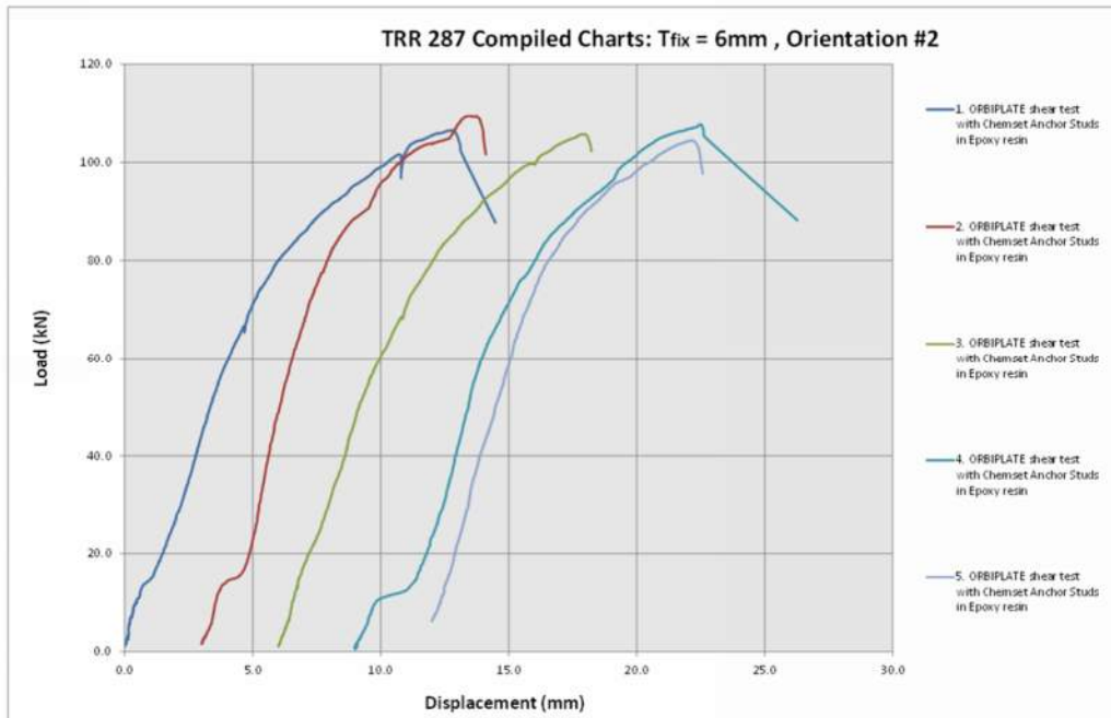
Shear Load vs Displacement Curve ORB2020PIAGH Rotational Horizontally aligned and bolt at extremity of slot 32mm plate thickness, M20 ChemSet Anchor Stud
