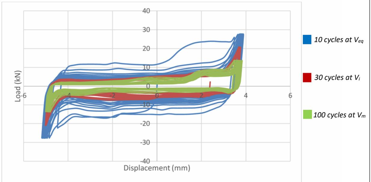
**Cyclic Loading for ORB2020BGH Longitudinal Vertically aligned upwards bolt central
